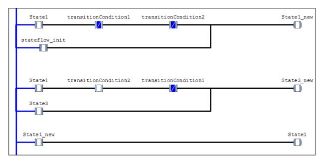
In the preceding Ladder Diagram, each rung of the ladder ends in a coil. The coil corresponds to a state of the original chart. The contacts before the coil determine if the coil receives power. You can compare the Ladder Diagram visually with the Stateflow chart. For instance, the coil State1 new receives power in one of these two cases:
