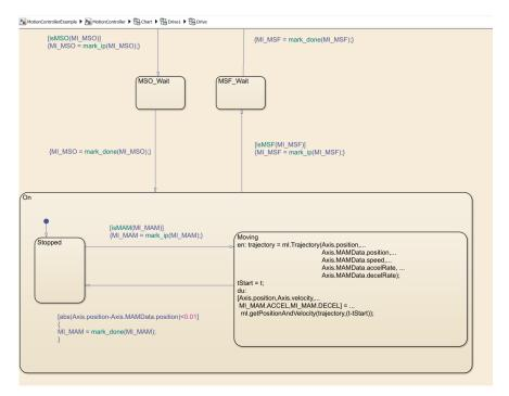
The drive logic Stateflow chart models a real world drive with parameters such as trajectory and delay. Any drive subchart has the following data:
