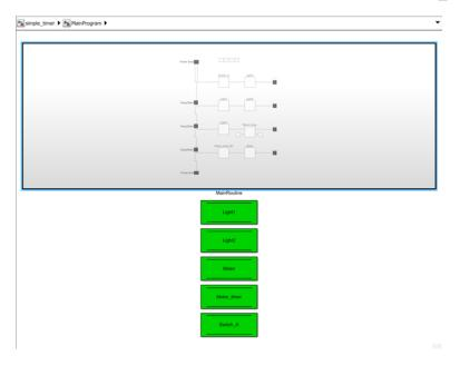
The MainRoutine subsystem contains the Simulink implementation of the simple\_timer.L5X Ladder Diagram. The ladder rung executes from top to bottom and left to right.
